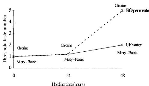
**Figure 6** Impact of holding time for T&O occurrence on UF and RO treated waters
