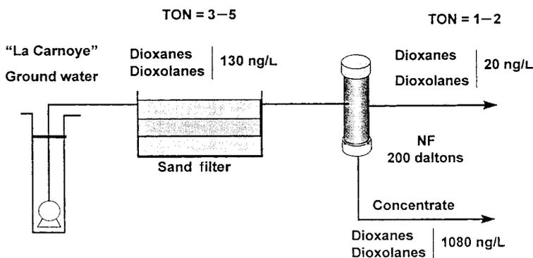
**Figure 3** Example of TON reduction using NF filtration
