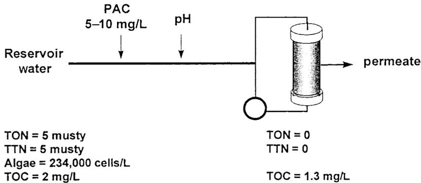
**Figure 2** Example of full-scale application, Apié plant, 28,000 m<sup>3</sup>/d
