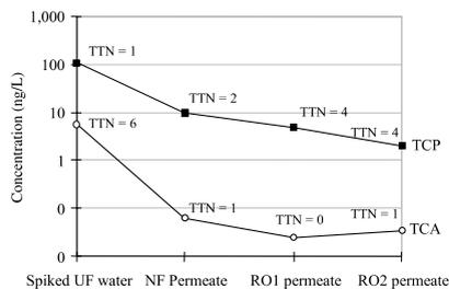
**Figure 5** TCA and TCP removal by NF RO membranes
