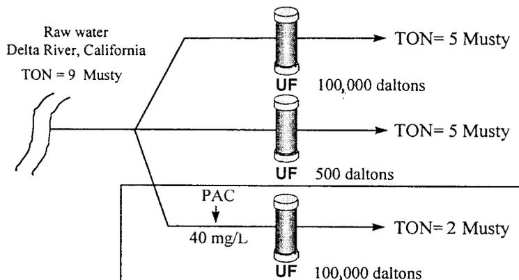
Figure 1 Impact of membrane cutoff on odour removal
